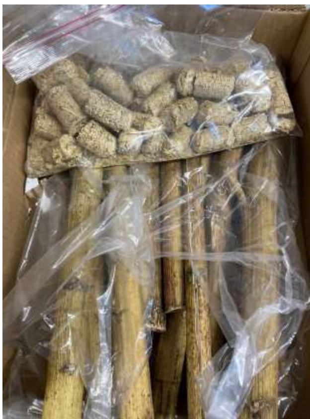
Figure 53: Residues from sunflower plant and briquettes from dried sunflower residues
