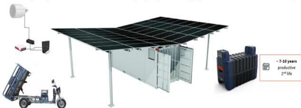
Figure 4: Representation of the containerised off-grid solar energy system
