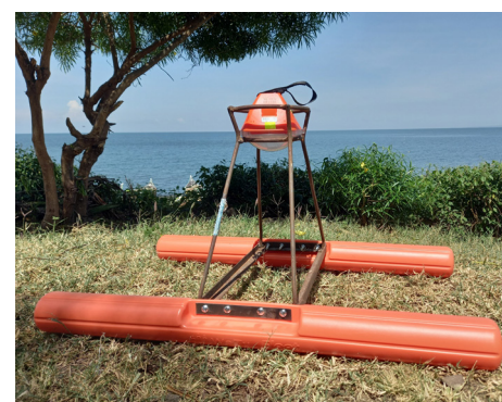
Figure 6: Solar powered night fishing lantern on a WeTu designed float (WeTu, 2023)
