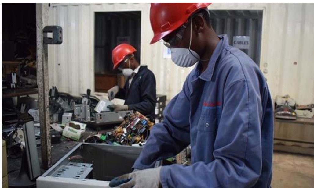
Figure 2: Dismantling of computers at WEEE Centre in Nairobi, Kenya (TNO Netherlands, 2022)
