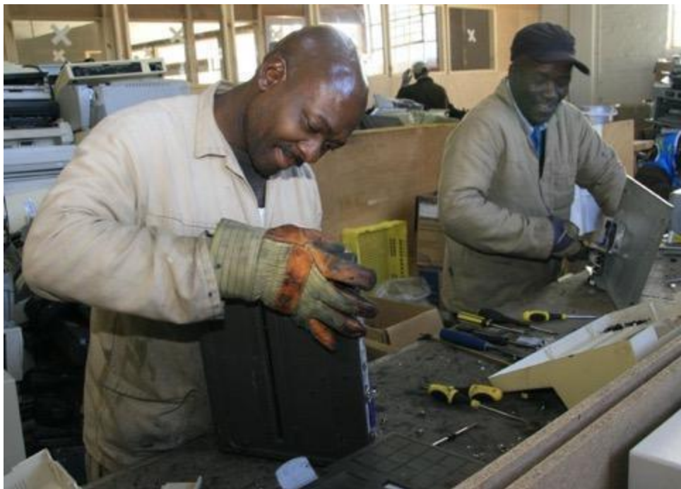
Figure 18. Manual dismantling of e-waste (Sustainable Recycling Industries, 2022)
