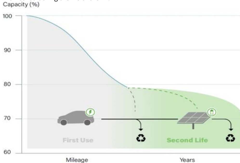
Figure 12. Second life for former EV batteries in stationary energy storage (Falk et al., 2020)
