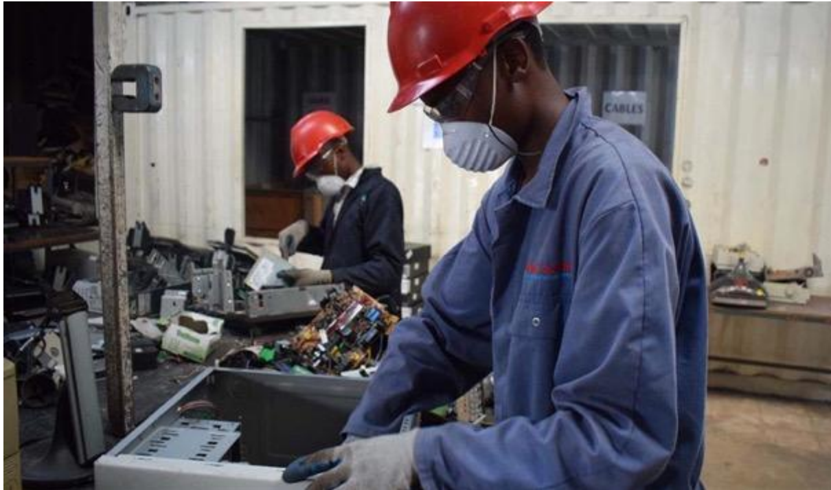
Figure 29. Dismantling of computers at WEEE Centre in Nairobi, Kenya (TNO, 2022)
