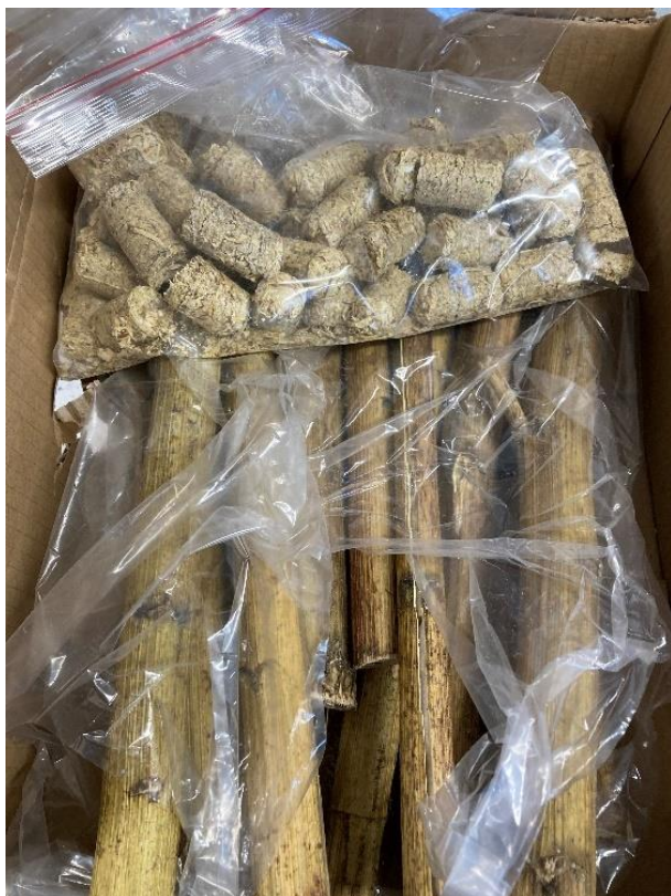
Figure 54: Residues from sunflower plant and briquettes from dried sunflower residues
