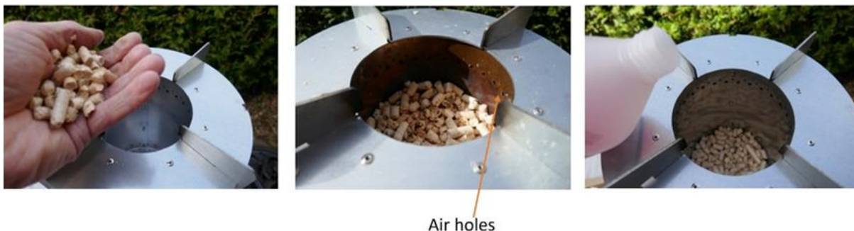
Figure 9: How to fill the fuel, Make it Green Solutions AB
