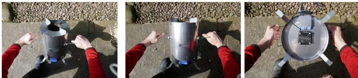
Figure 11: How to stop fire on MiG BioCooker, Make it Green Solutions AB
