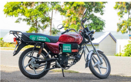
Figure: Converted Bajaj 100 from ICE to e-bike
