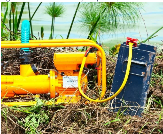
Figure 43: Ennos 2.0 HP pump with lithium ion battery pack during pilot test phase
