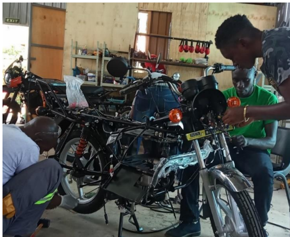
Figure 10: Bajaj 100 ICE bike conversion into e-bikes at WeTu's Technical Centre
